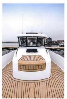
EcoDeck® is a strong, flexible, solvent free, UV-proof and polyurethane resin based flooring system. This prefabricated, viscous-elastic composite material has a stylish and warm effect, a seamless and durable finish and is suitable for numerous applications. It has a luxurious maritime effect.
